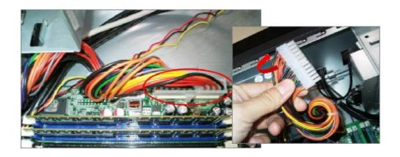
5.5 Pulling in Audio/FRONT USB/TOP USB/ CARD READER /FRONT cable to MB and put in cable clip
